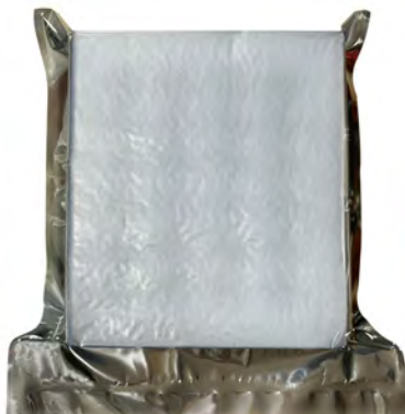
Seal the Tray with Anti-Static Bag
